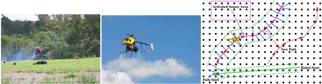
Figure 1: (Left) Helicopter in the air over the sensor network consisting of 54 Motes [10, 11]. The Motes sit on top of the dark flower pots. (Center) Helicopter. (Right) A sensor network with a path marked by sensor nodes. In response to an environment trigger, the sensor network computes a new path for the helicopter and an intermediate path to guide the helicopter to the new path.
