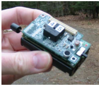
Figure 4: A Mica Mote with sensor board and long range antenna.
