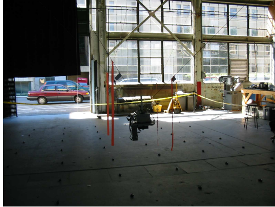
Fig. 2. The experimental testbed consisting of 49 Motes on the ground and the flying robot.
