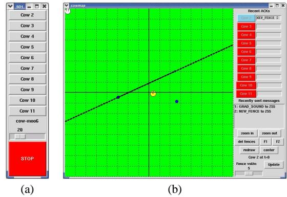
**Figure 2:** GUIs used on laptops to monitor field experiments. (a) Sound control GUI. Pressing a button triggers a sound on a specific cow. (b) Map control GUI. Shows the last reported position of each cow, whether it is currently playing a sound, and whether an Alive message has been received recently.
