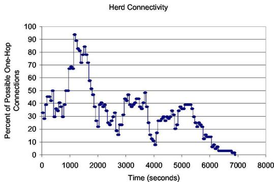
**Figure 4: Connectivity among the herd, measured by the percentage of one-hop connections present relative to all pairs of cows. At the beginning of the experiment, the cows were tightly clustered, so that most collars could communicate directly with most others. In the field, the connectivity was less complete but still sufficient and fairly consistent.**
