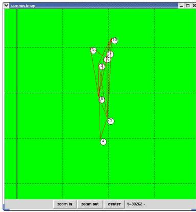
**Figure 3: Network connectivity among the herd at one point in time during field experiments. It can be seen that many connections exist, but even some short ones do not, presumably due to the locations of the antennas relative to the animals' bodies and the ground.**
